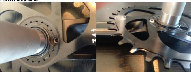
3. Mounting the chainring backwards with the logo side out will not allow the bolt to sit at its proper, countersunk, height and may cause damage to the chainring and BB when installed.
